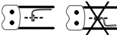
FIGURE 1a: SENSOR AND MAGNET INSTALLATION (Sensor Installed on Centerline of Seat)
