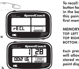
To recall the memory hold down the top button for 2 Seconds until "rECL" appears in the bottom left-hand window (a). At this point, release the button and the first memory point will appear (b).
