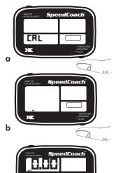
To select and change the units which your unit will display, press and hold the lower button. After 3 Seconds, the unit will pass through the calibration mode(a) and scroll through each available unit (b). When your desired unit appears in the lower left window, release the button (c).
